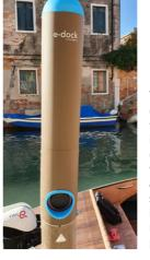
The engineering definition of the upper part is the result of collaboration with ORVIM S.r.l., a local company specializing in composite materials and prototype design The boat used for the test phase in Venice was built by Edyn Marine Company, based on a project by the German nautical designer Kaiser. It is equipped with an 11 kW Edyn engine and a battery with a capacity of 8.5 kWh
